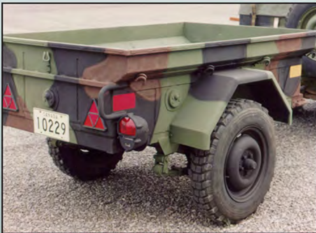
M101, 500 lbs capacity, over 2000 manufactured to date
