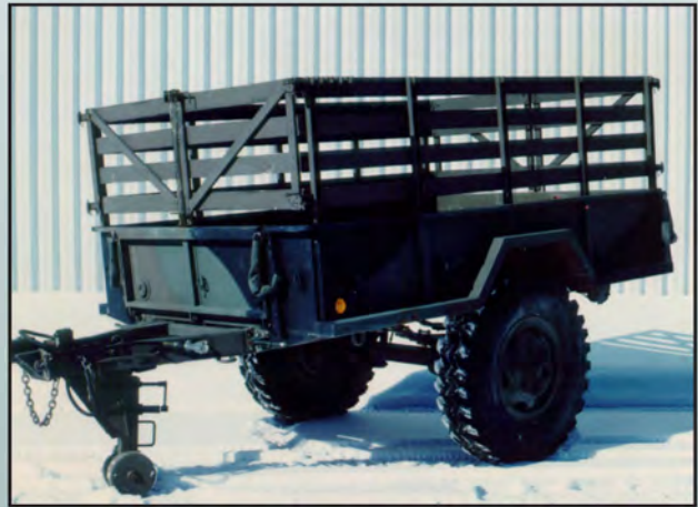
DEW Model 2910, 2000 lbs capacity, over 1500 manufactured to date
